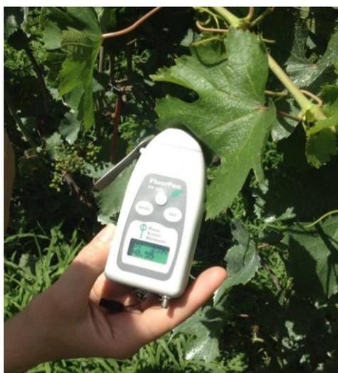
**Figura. 7:** Fluorimetro portatile FluorPen FP100 (Photon System Instruments, CZ).
